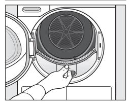
■ Pull the upper fluff filter forwards to remove it.
